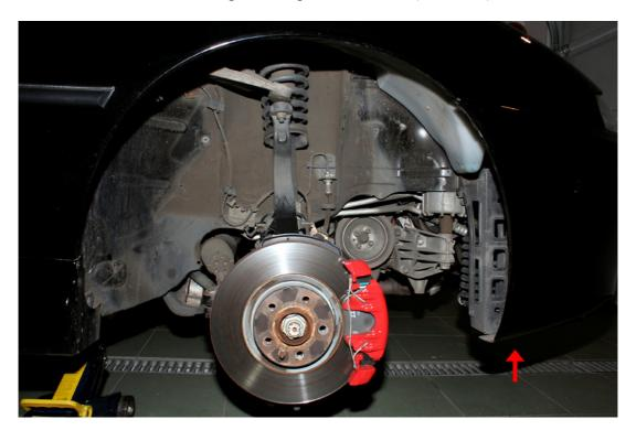
4. Working from under the wing remove the two bolts on the inner side of the bumper (red arrows).
