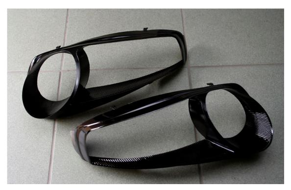
11. Install the painted plastic into the glass. Work in clean environment, as all dirt will be visible in your headlight when you seal it.
