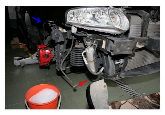
• Start removing the bumper. It should go very easy. Start on the side, from the wheel arch. There are two pins on each side holding the bumper. When the bumper comes off them, the rest is not difficult.
