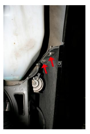
5. By now, you should have removed all five bolts from under the bumper. The three in the front (red arrows) you should have removed in step 1 with the under engine protection. The two on the sides you should have removed in the step 3.
